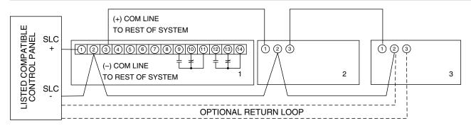
**Note:** For terminals 9 through 14, normally closed and normally opened relay positions are defined with product in reset condition, not in alarm.
